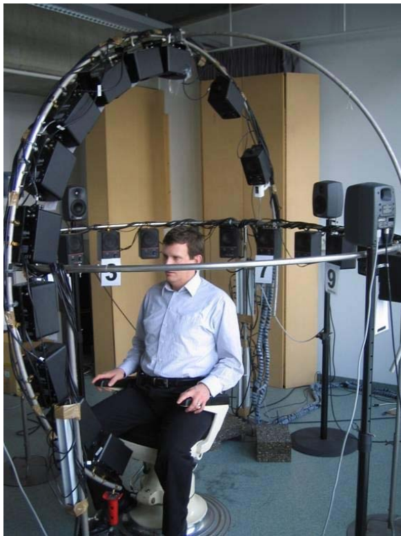
Figure 7. View of the test setup for left/right, elevation, and front/back localizations.
